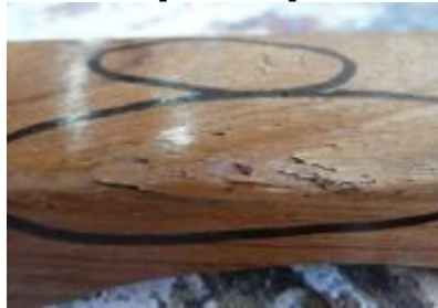
Corner edge of xylo bar has extreme splintering.
