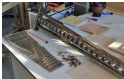
Removing the bars revealed years of deterioration on the bar rails and end caps.
