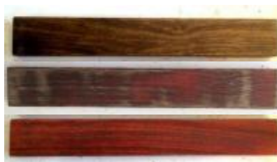
[Top] Sun-bleached surface [Middle] During sanding [Bottom] After Sanding
