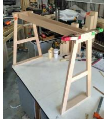
The accurate transferring of the old bar rail dimensions was crucial to ensure proper alignment of the resonators directly under the acoustic centers of the bars.
